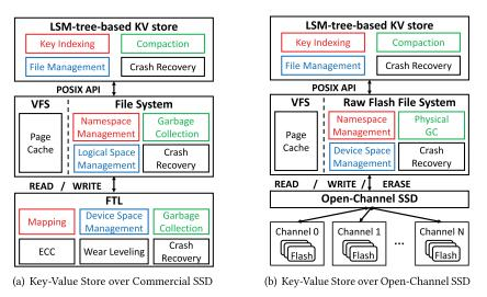
Fig. 2. KV Store Architectures on Flash Storage.
