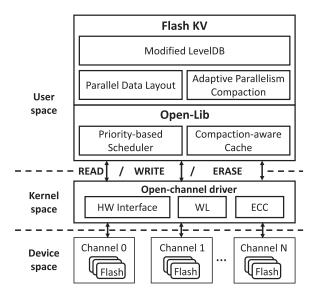
Fig. 3. The FlashKV Architecture.
