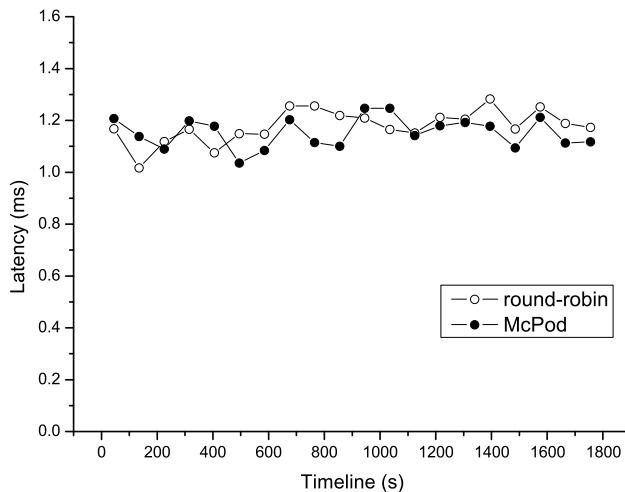
Fig. 14. Performance comparison between McPod layout and round-robin layout for the WebSearch2 workload after one scaling operation “4 + 1.”
