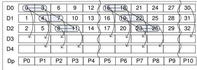
Fig. 2. Coalesced reads for RAID-4 scaling from four disks to six. Multiple successive blocks are read via a single I/O.
