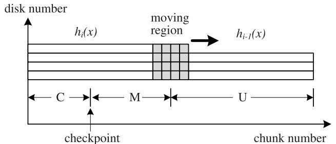
Fig. 7. Delayed updates of layout metadata. “C”: migrated and checkpointed; “M”: migrated but not checkpointed; “U”: not migrated. Data redistribution is checkpointed only when a user write request arrives in the area “M”.
