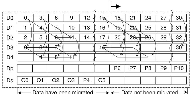
Fig. 5. All parity updates brought by RAID scaling are outsourced to a surrogate disk,  $D_s$ .
