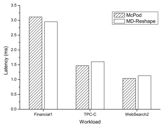
Fig. 17. Performance comparison between McPod layout and round-robin layout for different workloads after two scaling operations “4 + 1 + 1.”
