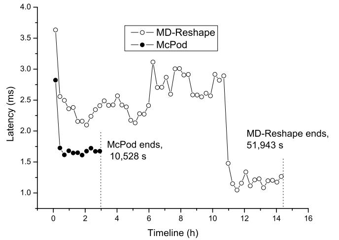
Fig. 13. Performance comparison between McPod and MD-Reshape for the TPC-C workload.
