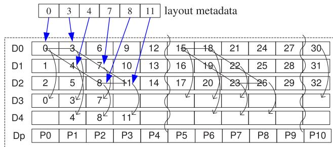
Fig. 6. If data blocks are copied to their new locations and metadata are not yet updated when the system fails, data consistency is still maintained, because the data in their original locations are valid and available.
