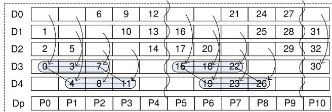
Fig. 3. Coalesced writes for RAID-4 scaling from four disks to six. Multiple successive blocks are written via a single I/O.
