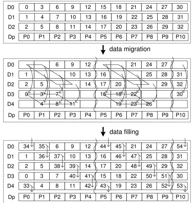
Fig. 1. RAID-4 scaling from four disks to six using McPod.
