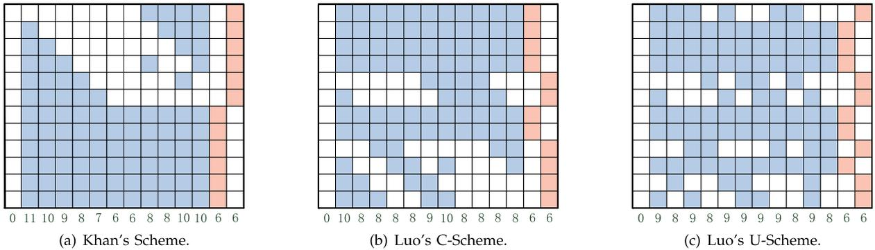
Fig. 4. An recovery example of 14-disks Blaum-Roth code under different recovery schemes when the first disk failed (The blue squares mean the data elements that require to be accessed, while orange squares indicate the parity elements that need to be read).
