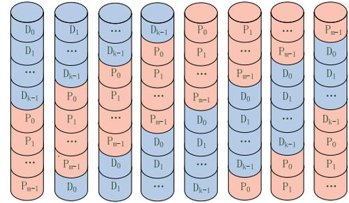
Fig. 3. A widely used case of one stack in practical erasure coded storage systems.
