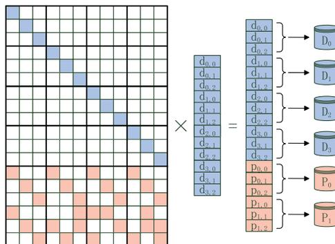
Fig. 2. An example of generator bitmatrix of Cauchy Reed-Solomon code with  $n = 6$ ,  $k = 4$ ,  $m = 2$ , and  $w = 3$ .
