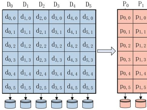
Fig. 1. An example of one stripe in erasure coded storage systems, where  $n = 8$ ,  $k = 6$ ,  $m = 2$ , and  $w = 6$ .
