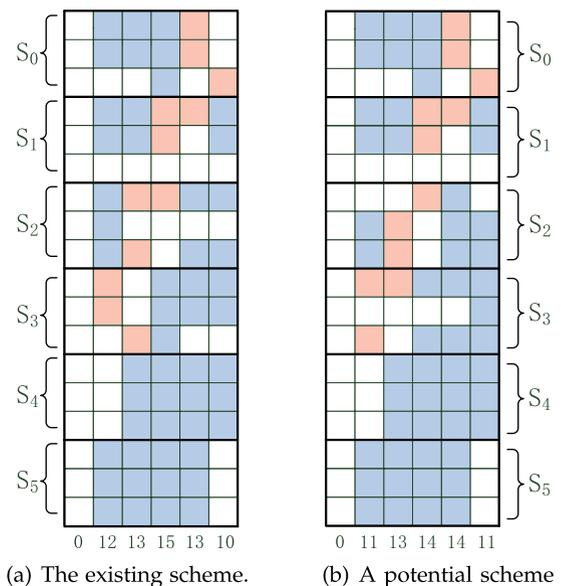
Fig. 5. A recovery example in stack-level when the first physical disk failed ( $S_i$  means the  $i$ th stripe,  $0 \leq i \leq 5$ ).
