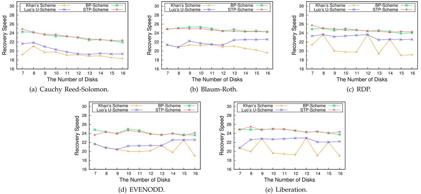
Fig. 7. The recovery speed over different erasure codes with  $m = 2$  (Unit: MB/s).
